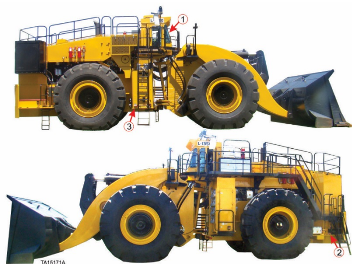
Figure 29. Locations of fire suppression system actuation switches (typical locations - standard installation)
