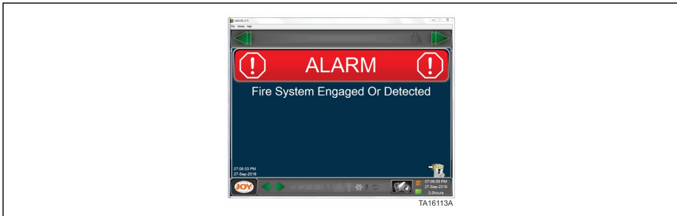
Figure 21. Fire suppression system engaged or detected red alarm screen
